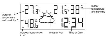
\* When the signal is successfully received by the weather station, the outdoor transmission icon will be switched on. (If not successful, the icon will not be shown on LCD). The user can then easily see whether the last reception was successful (icon on) or not (icon off).
